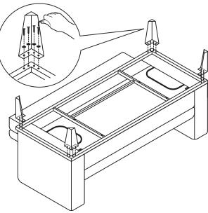
**5** Align the holes on the support leg onto the pre-drilled holes on the base frame as shown below, secure with two long bolts and small washers by provided allen key.
